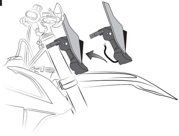
**Connect the power cables and mount the Acerbis headlight to the bike using the original rubber mounting bands.**
