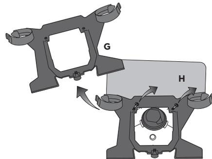
**Remove the screws (H) and the frame (G) from the original headlight mask.**
