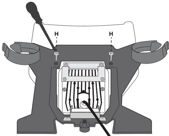
**Attach the frame (G) to the headlight (A) using the original screws (H).**
