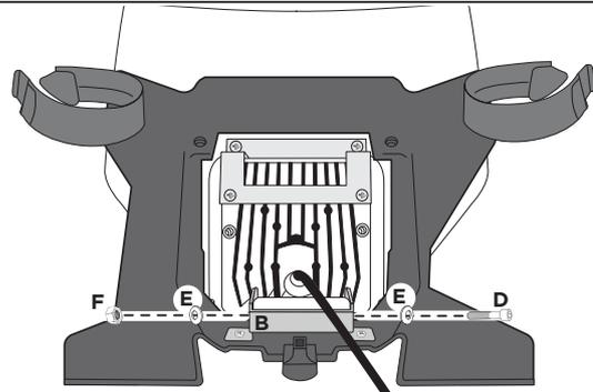
**Attach the Acerbis headlight (A) to the original frame using the screw (D), the washers (E) and the nut (F) through the bracket (B).**
