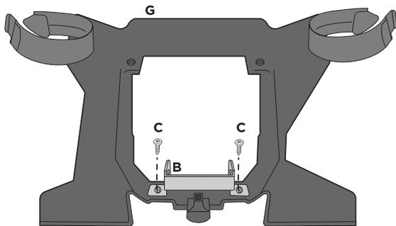
**Assemble the bracket (B) on the original frame (G) using the screws (C).**
